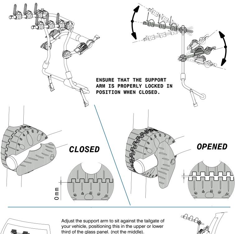
The carrier should lean towards your vehicle maintaining approximately 8 cm (3 inches) clearance from the car bodywork. If this is not the case, open the adjuster handles and reposition.
